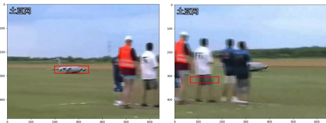
Fig. 6: SiamFC failed to track toyplane after occlusion
